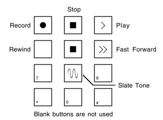
Figure 4.4; Keypad assignments for soundbite recorder
