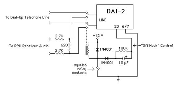
Figure 3.5; Using both and RPU and telephone line with the DAI-2
