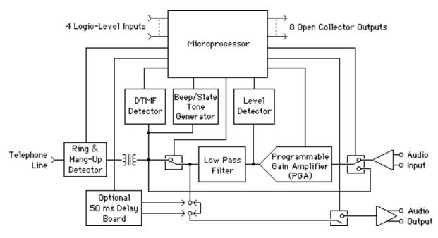
Figure 6.1; DAI-2 block diagram
