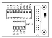
Figure 3.3; Relay Panel connects at J1
