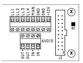
Figure 4.3; Relay panel connections
