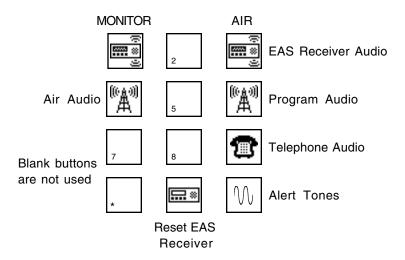
Figure 4.6; Key assignments for Emergency Broadcast Operation
