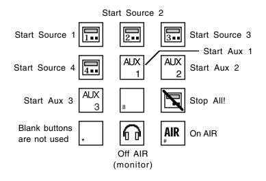
Figure 4.5; Keypad assignments for remote broadcaster
