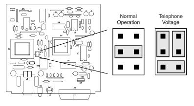
Figure 4.2; Telephone voltage jumpers JP1
