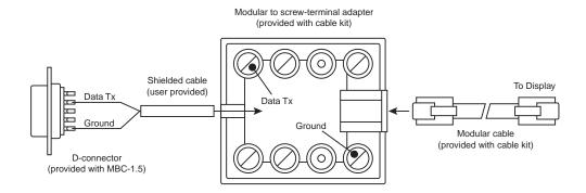
The Beta-Brite has a modular connector that does not accommodate shielded cable. A short RJ-12 cable and an RJ-12 to screw-terminal adapter are included in the cable kit. These form a simple and reliable connection between the shielded cable run and the modular jack on the Beta-Brite.
