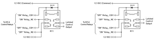
Note: This circuit "powers up" with the latched output "ON."
