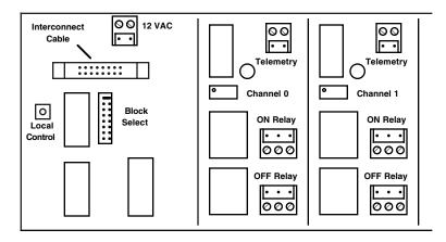
Each RP-8 panel has a movable "Block Select" jumper plug which is used to select the block of channels assigned to that panel. The blocks are: 0-7, 8-15, 16-23, 24-31, 32-39, 40-47, 48-55, and 56-63. There is also a "Local Control" pushbutton, accessible from the front of the panel, which allows all control and telemetry functions to be accessed from the local telephone.
