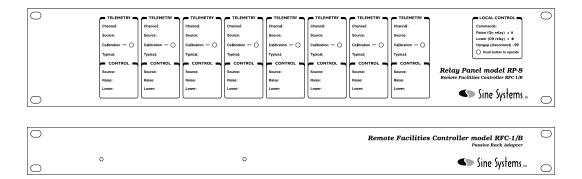
The cable included with the RFC-1/B system has one connector at each end. If this is a new installation with a single RP-8 relay panel, attach the flat cable to the RFC-1/B at one end and the RP-8 at the other.
