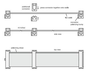
Make sure that the connector is aligned directly across the cable. If the connector is at an angle, the metal teeth on the connector may penetrate the cable insulation at the wrong points and short the conductors or miss them entirely.
