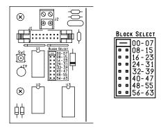
Each relay panel should operate on a different channel block. Blocks are usually used continuously from channel 00 up but a block of channels may be skipped if necessary.
